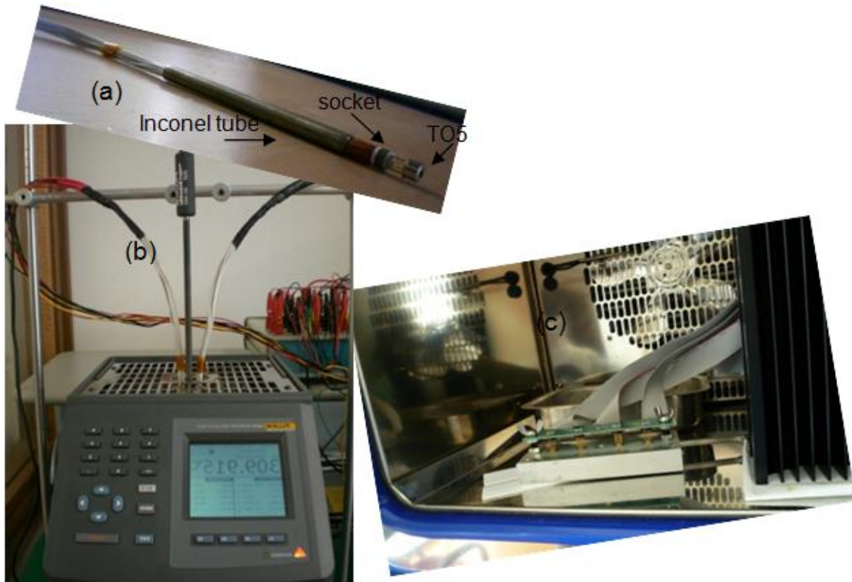
Fig. 4 Measurement set-up for isothermal calibration. (a) Probe for measurement in the Metrology Well. From the right to the left: the TO-5 package; the Teflon socket and the Inconel tube; (b) Metrology well; (c) close up of the CTS T-65/50 oven inside. The top part of the TO5 packages, where the chips are glued, are inserted in an Al block and the temperature is measured with a PRT thermometer.
