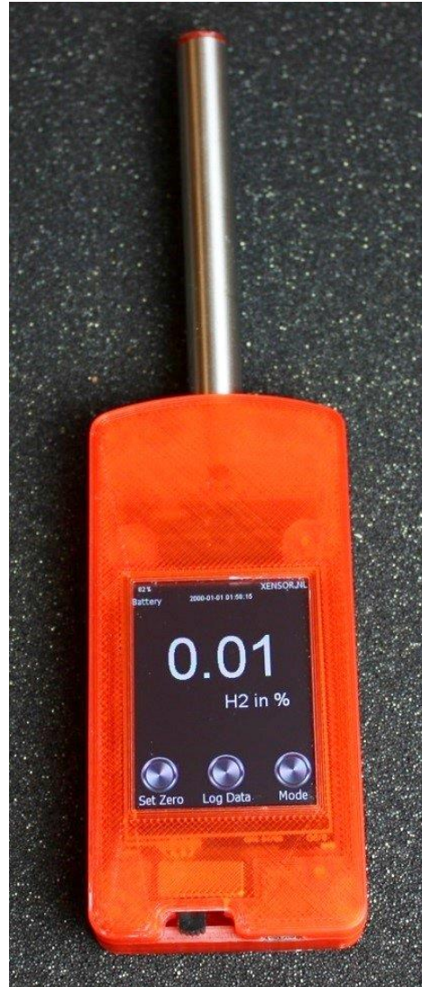
XEN-5320-D handheld sensor (210 x 54 x 19 mm)
